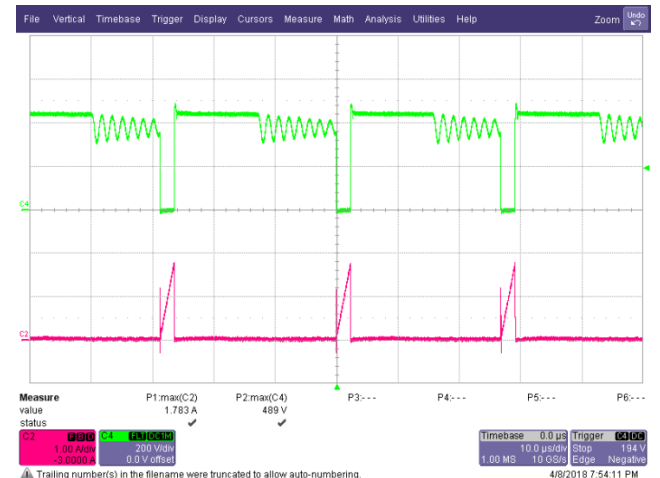
Figure 38 – Drain Voltage and Current Waveforms. 265 VAC, 9.0 V, 3 A Load, (489 V MAX ). Upper: V_{DRAIN} , 200 V / div. Lower: I_{DRAIN} , 1 A / div., 10 \mu s / div.
