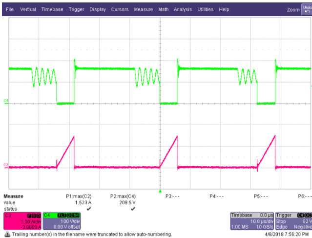
Figure 35 – Drain Voltage and Current Waveforms. 90 VAC, 5.0 V, 3 A Load, (209.5 V MAX ). Upper: V_{DRAIN} , 100 V / div. Lower: I_{DRAIN} , 1 A / div., 10 \mu s / div.
