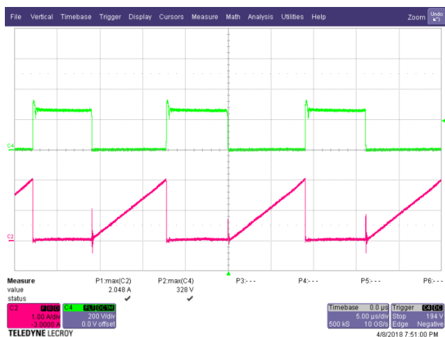
Figure 41 – Drain Voltage and Current Waveforms. 90 VAC, 20 V, 3 A Load, (328 V_{MAX} ). Upper: V_{DRAIN} , 200 V / div. Lower: I_{DRAIN} , 1 A / div., 5 \mu s / div.
