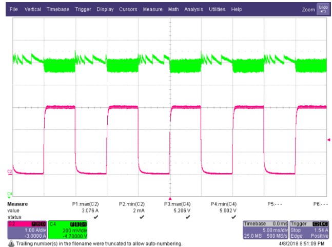
Figure 28 – Transient Response. 265 VAC, 5.0 V, 0 – 3 A Load Step. V MIN : 5.002 V, V MAX : 5.206 V. Upper: V OUT , 0.2 V / div., 5 ms / div. Lower: I LOAD , 1 A / div.
