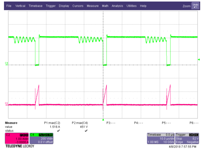
Figure 36 – Drain Voltage and Current Waveforms. 265 VAC, 5 V, 5 A Load, (451 V MAX ). Upper: V_{DRAIN} , 200 V / div. Lower: I_{DRAIN} , 1 A / div, 10 \mu s / div.
