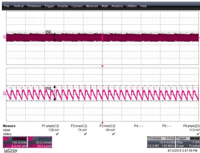
Figure 63 – Output Ripple.(pk-pk – 128 mV) 90 VAC Input, 20.0 V, 3 A Load. V_{OUT} , 100 mV / div., 10 ms / div.
