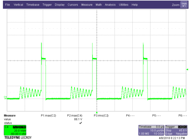
Figure 46 – SR FET Voltage Waveforms. 265 VAC, 9 V, 3 A Load, (88.1 V MAX ). C4: SR_V DRAIN , 20 V / div., 10 μs / div.
